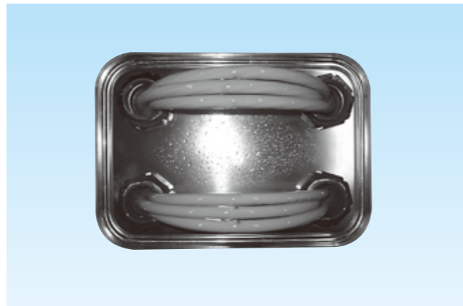
Condition of cables right after soaked in coolant
