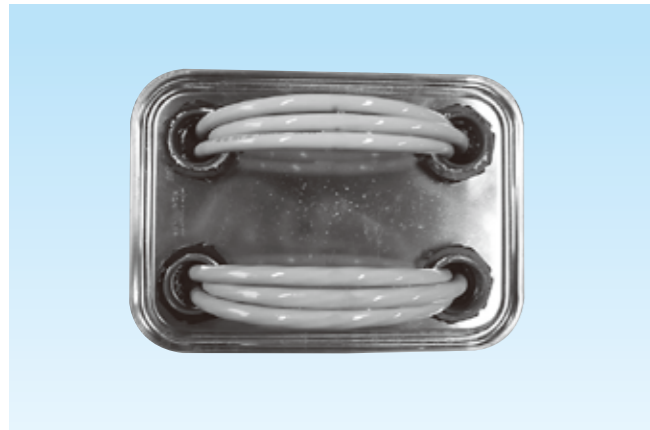
Condition of cables being soaked in coolant
